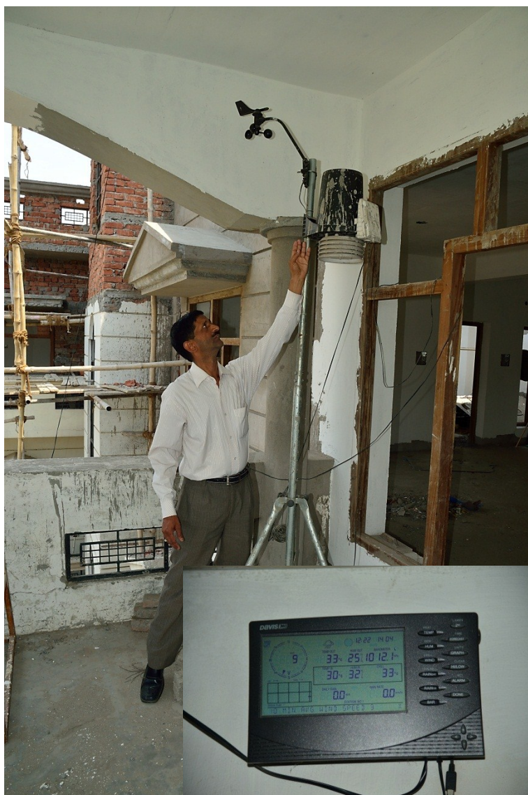
The automatic weather station (temporarily relocated) being explained by Kailash Pandey, GEAG Climatologist (with the readout, bottom RHS)
